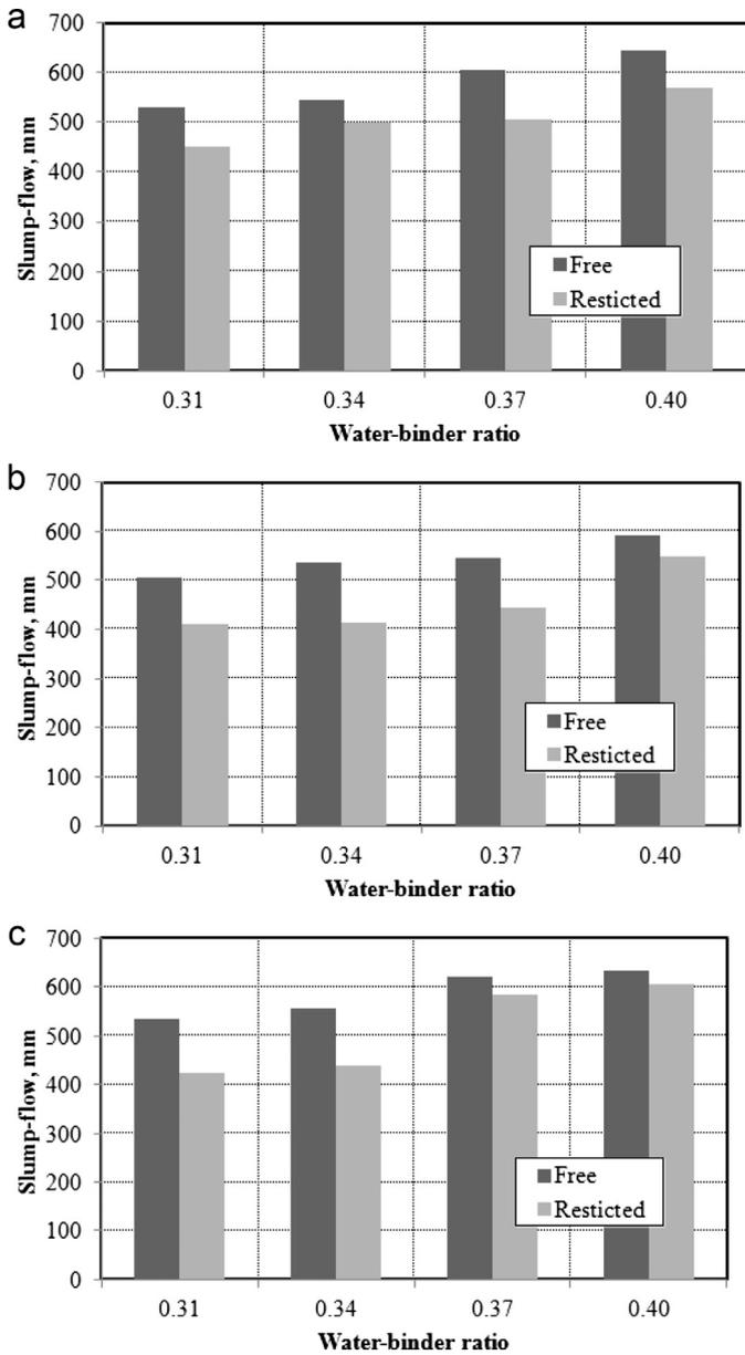
Fig. 5. a. Free and limited slump-flow of SCC with LS. b. Free and limited slump-flow of SCC with RA. c. Free and limited slump-flow of SCC with MW.
