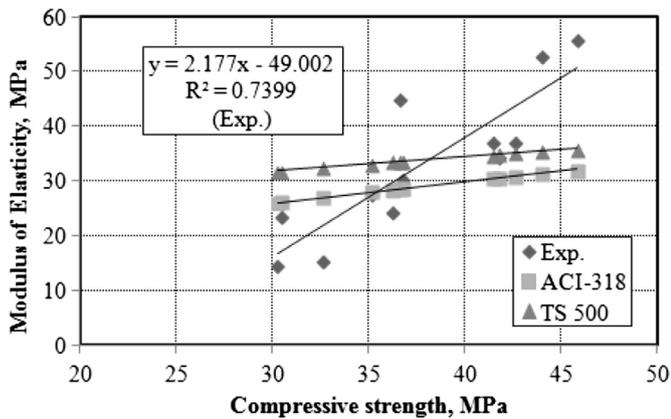
Fig. 12. The relationship between E-moduli and compressive strength.
