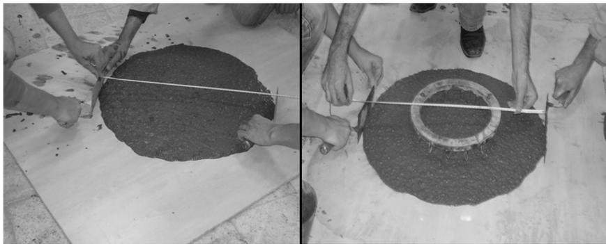
Fig. 1. Free and restricted slump-flow.
