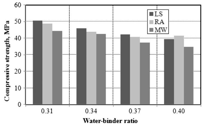
Fig. 7. Comparison of compressive strength of 7 aged specimens.
