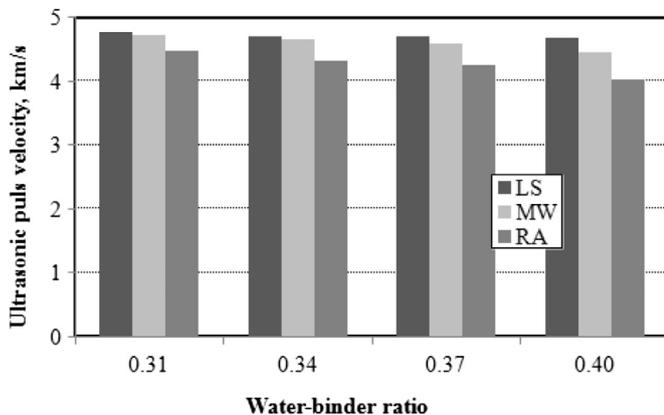
Fig. 13. Comparison of ultrasonic pulse velocity of the SCC series.
