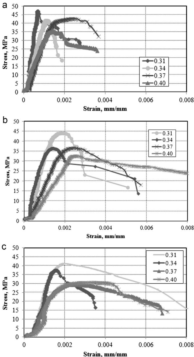
Fig. 10. a. Stress-strain curves for LS series. b. Stress-strain curves for RA series. c. Stress-strain curves for MW series.
