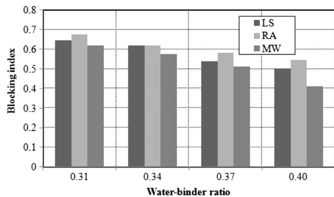
Fig. 6. Blocking index of SCC with different type of aggregates.
