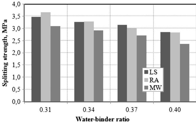
Fig. 9. Comparison of splitting tensile strength of 28 aged specimens.
