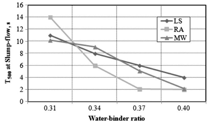
Fig. 4. Time to  $T_{500}$  during the slump-flow test.
