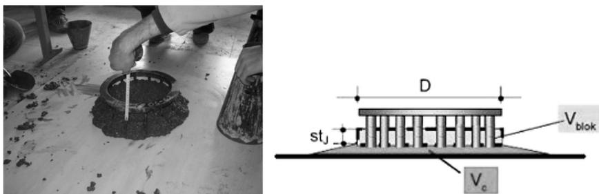
Fig. 2. Measurement of blocking concrete in J-ring.
