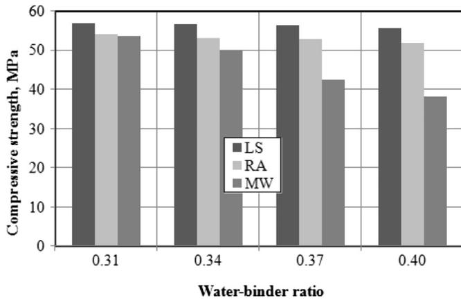
Fig. 8. Comparison of compressive strength of 28 aged specimens.
