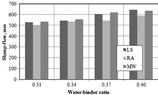
Fig. 3. Slump-flow test on SCC with different type of aggregates.
