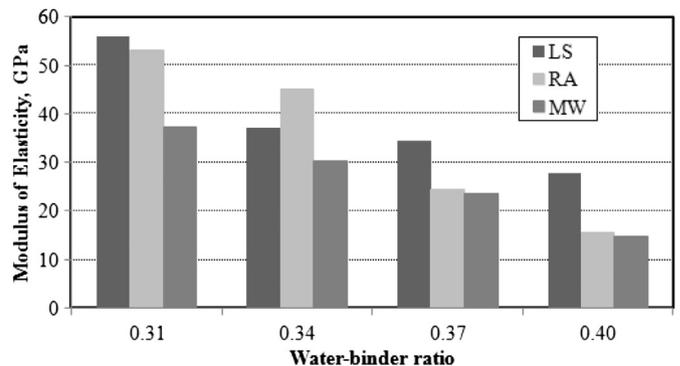
Fig. 11. Comparison of modulus of elasticity for SCC series.
